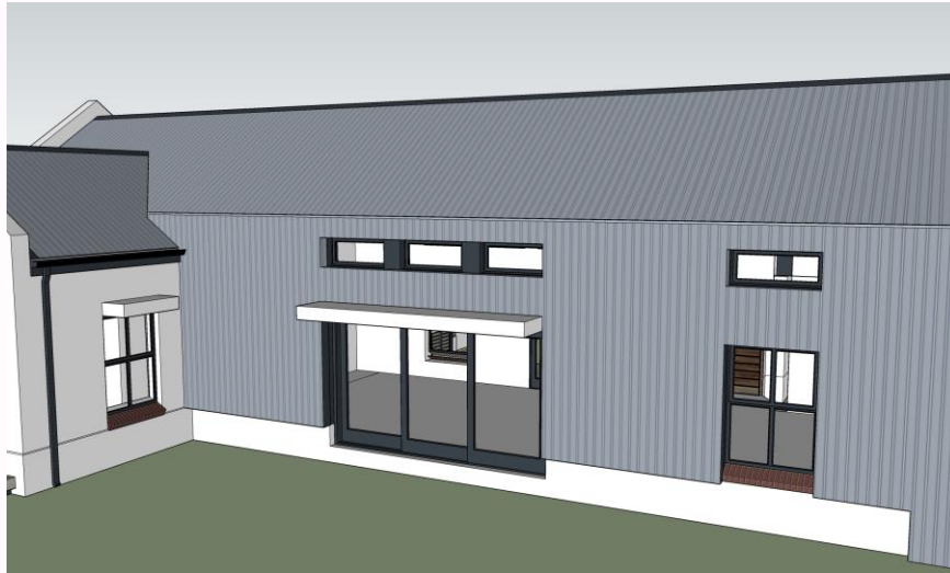
Clearstory windows in cladded wall are permitted without eyebrows in a single storey dwelling.
