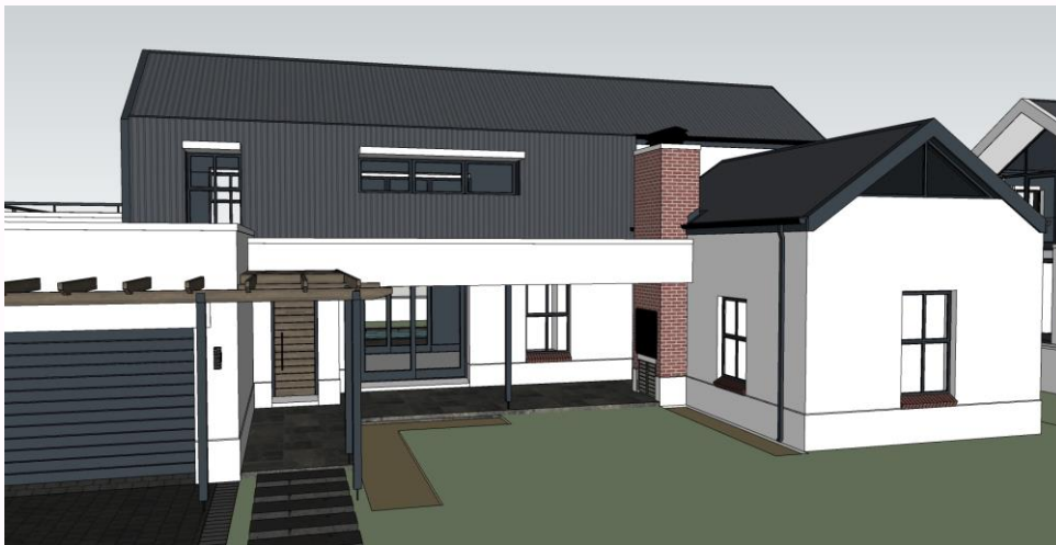
All windows within vertical side cladding must have eyebrows.
