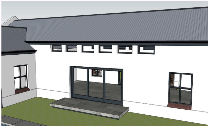
Clearstory windows in plastered wall (Single storey)
