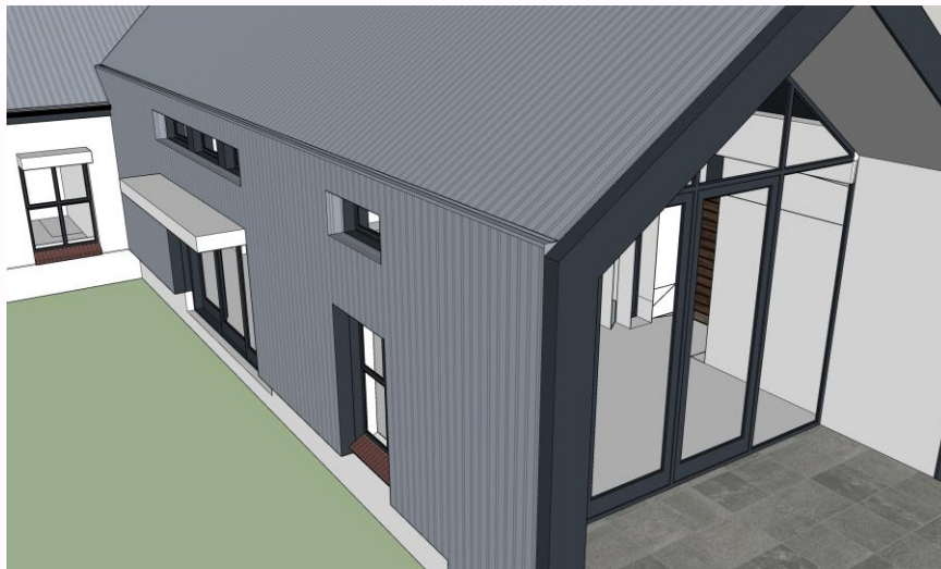
Concealed gutter behind cladding
